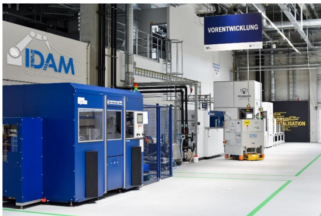
Image 1: IDAM (Industrialization and Digitization of Additive Manufacturing) has set up the digitally networked, fully automated 3D printing production line and fully integrated it into automotive series production. © BMW Group.
