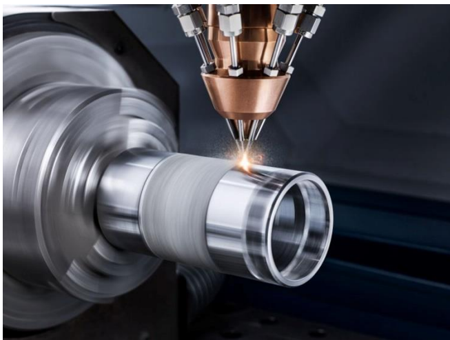
Image 1: Extreme high-speed Laser Material Deposition EHLA with innovative TRUMPF system technology. © TRUMPF GmbH + Co. KG (Holding), Ditzingen, Germany.
