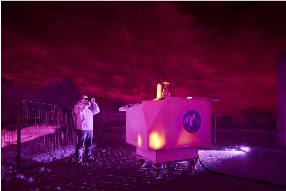
Image 6: The mobile LIDAR system sends five beams into the night sky. With four small and one large telescope, it detects the photons from up to 100 km altitude and provides climate data in real time. © Fraunhofer ILT, Aachen, Germany / Ralf Baumgarten.
