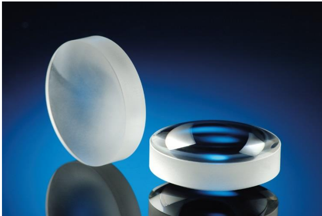
Image 1: Laser-polished sphere made out of BK7. © Fraunhofer ILT, Aachen, Germany.
