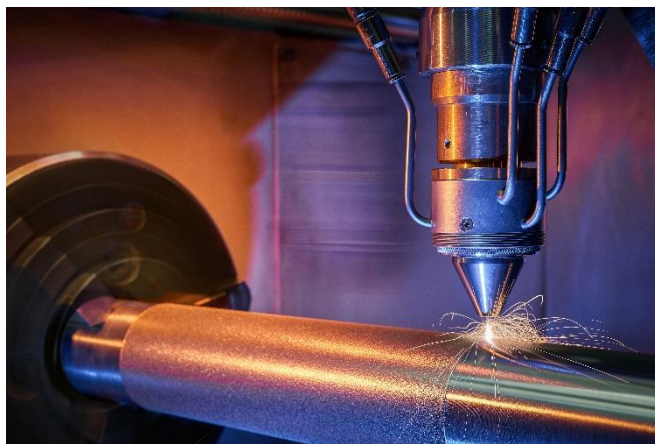
Image 3: EHLA can be used to apply protective metal coatings at extremely high speeds. © Fraunhofer ILT, Aachen, Germany / Volker Lannert.
