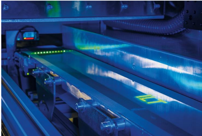
Image 3: A complex process: the ablation of nanometer-thin layers on a moving film with USP laser scribing in the fs regime. © Fraunhofer ILT, Aachen, Germany / Volker Lannert.
