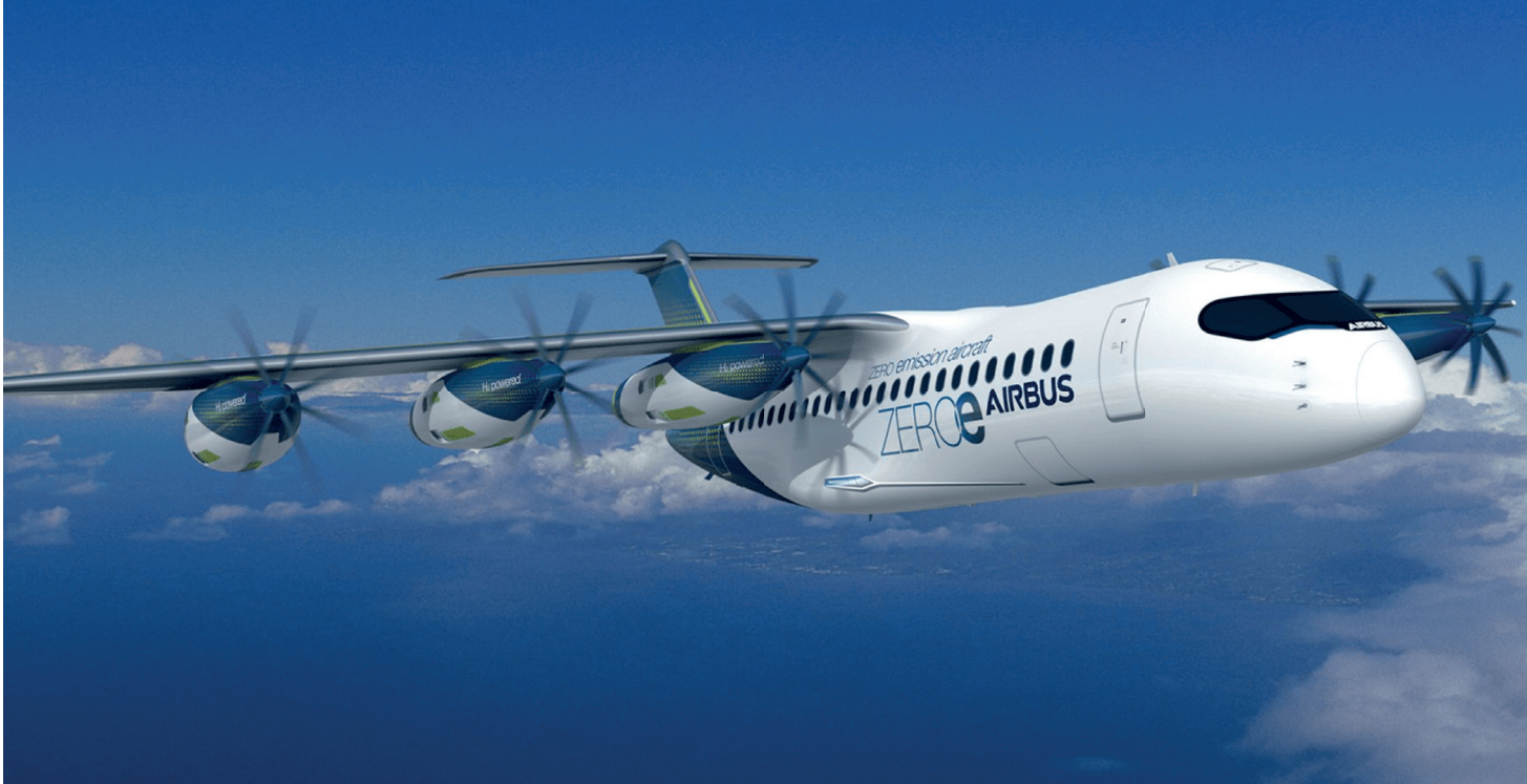
All-electric concept aircraft powered by fuel cells, © Airbus Group.
